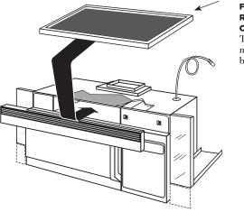
FILTER KIT JX81D-RECIRCULATING CHARCOAL FILTER KIT To be used when the microwave oven cannot be vented to the outside.
